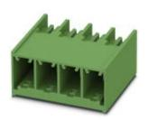
PCB headers, nominal current: 41 A, number of positions: 2, pitch: 7.62 mm, color: green, contact surface: Tin, mounting: Wave soldering
