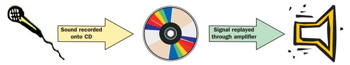
The major sections in this system are essentially translators. They take a signal in one form and put it into another. In the end, the sound signal is translated back into its original form, a physical sound wave.
