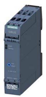
Thermistor motor prot. relay Standard evaluation unit 22.5 mm enclosure Screw terminals 2 CO contacts, bistable US = 24 V-240 V AC/DC Manual/Auto/Remote RESET 2 LEDs (READY/TRIPPED) Galvanic separation Test/Reset button Open-circuit monitoring Short-circuit monitoring Non-volatile
