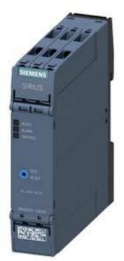
Thermistor motor prot. relay Device for warning and tripping 22.5 mm enclosure Screw terminals 1 NO contact + 1 CO contact US = 24 V-240 V AC/DC Manual/Auto/Remote RESET with ATEX certification 3 LEDs (READY/WARNING/TRIPPED) Protective separation Test/Reset button Open-circuit monitoring Short-circuit monitoring Non-volatile 2 separate PTC sensor circuits
