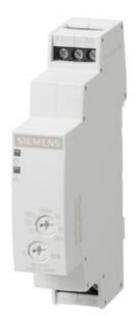
TIME RELAY, MOUNT. ON-DELAY 1 W, 7 TIME SETTING RANGES, 0.05 S...100 H, AC/DC 12. .240 V, WIDE RANGE SUPPLY VOLTAGE
