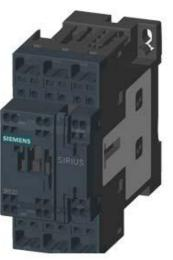
CONTACTOR, AC-3, 4KW/400V, 1NO+1NC, AC(50-60HZ)/DC ACTUAT. AC/DC 200...280V, 3-POLE, SZ S0 SPRING-LOADED TERMINAL
