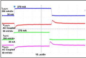
**FIGURE 2-21:** LDO1, LDO2 Load Transient Response.
