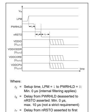
FIGURE 4-9: Entering Hibernate Mode Timing Diagram.
