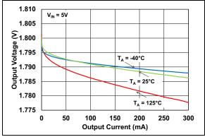
**FIGURE 2-12:** LDO2 Output Voltage vs. Output Current and Temperature (V<sub>LOUT2</sub> = 1.8V).
