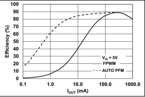
FIGURE 2-6: Buck3 Efficiency vs. Load Current ( $V_{OUT3} = 1.25V$ ).
