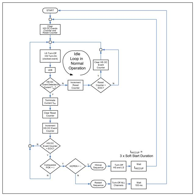
FIGURE 5-2: Hiccup Mode Protection Flowchart.
