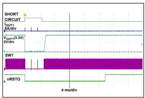
FIGURE 2-20: Output Short Circuit on  $V_{OUT1} - HCPEN = 1$ .
