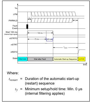
FIGURE 4-11: Automatic Wake-up Pulse Generation Timing Diagram (Fault during Hibernate).
