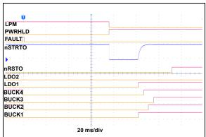
FIGURE 2-24: Automatic Wake-up Pulse, Hibernate Mode.
