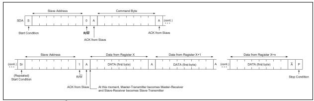
FIGURE 4-15: I<sup>2</sup>C Block Read.
