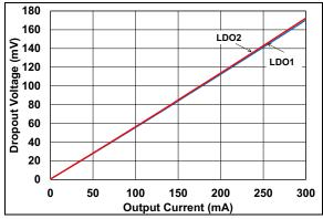
FIGURE 2-13: LDO1, LDO2 Dropout Voltage vs. Load Current.
