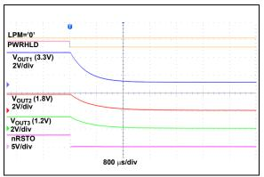
**FIGURE 2-16:** PWRHLD Shutdown Sequence.
