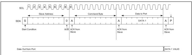
FIGURE 4-12: I<sup>2</sup>C Single Write.
