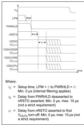
**FIGURE 4-7:** Power-Down (Shutdown) Sequence Timing Diagram.
