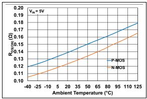
**FIGURE 2-10:** MOSFET  $R_{DS(ON)}$  vs. Temperature.
