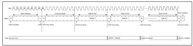
FIGURE 4-13: Block Write.
