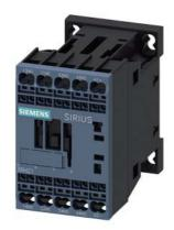
Coupling contactor relay, 3 NO + 1 NC, 30 V DC, 0.7 ... 1.25\* US, with integrated diode, Size S00, Spring-type terminal suitable for PLC outputs
