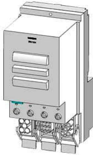
ET 200PRO ERSE/RSSE HF ELEKTRONISCHER REVERSIERSTARTER ELEKTRONISCH (SANFT-) SCHALTEN MOTORVOLLSCHUTZ BESTEHEND AUS: ELEKTRO. UE-SCHUTZ + THERMISTOR 3 AC 400V/5,5KW; 1,5A...(9A)12A OHNE BREMSKONTAKT 4DI HAN Q4/2 - HAN Q8/0
