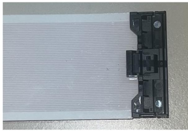
White jacket is pulled back so no interference with clips. This will call a small about of the shield to be exposed at the edge of the clips as seen above.
