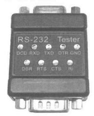
72-9200 is RS-232 (DB9) cable tester. 72-9200 can test the "Open" & "Short" of RS-232 cable. It is standard DB9 male to DB9 female cable tester. 72-9200 use 9 pcs blue LED to show the test result.
