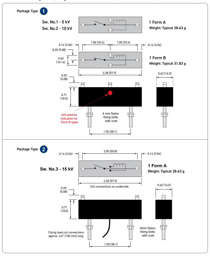
**Important:** For all Form B types, the correct coil polarity must be observed. The positive connection is shown by the red spot on the package.
