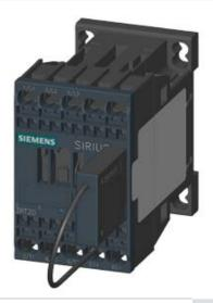
CONT. F. RAILW. A., AC-3, 5.5KW 400V, DC 24V, 0.7...1.25\*US, W.SUPPRESSORDIODE INTEGRATED, 3-POLE, SZ SO SPRING-LOADED TERMINAL FOR STANDING MOUNTING POSITION
