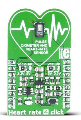
**Heart rate 4 click** carries the <u>MAX30101</u> high-sensitivity pulse oximeter and heart-rate sensor from Maxim Integrated.
