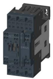
CONTACTOR, AC-3, 15KW/400V, 1NO+1NC, AC 24V 50HZ, 3-POLE, SZ SO SPRING-LOADED TERMINAL
