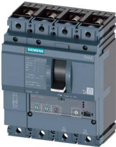
CIRCUIT BREAKER 3VA2 IEC FRAME 100 BREAKING CAPACITY CLASS M ICU=55KA @ 415 V 4POLE, LINE PROTECTION ETU320, LI, IN=25A OVERLOAD PROTECTION IR=10A ...25A SHORT CIRCUIT PROTECTION II=12 X IN NEUTRAL PROTECTION ADJUSTABLE(OFF,100%) BUSBAR CONNECTION
