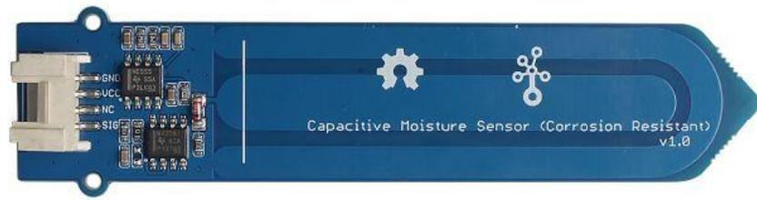
The Grove - Capacitive Soil Moisture Sensor (Corrosion Resistant) is a soil moisture sensor based on capacitance changes. Compared with resistive sensors, capacitive sensors do not require direct exposure of the metal electrodes, which can significantly reduce the erosion of the electrodes.
