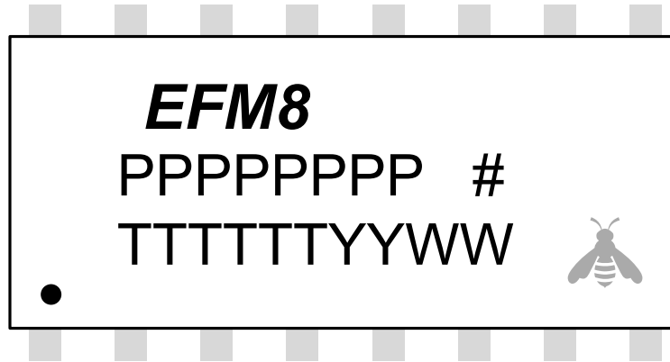
Figure 9.3. SOIC16 Package Marking
