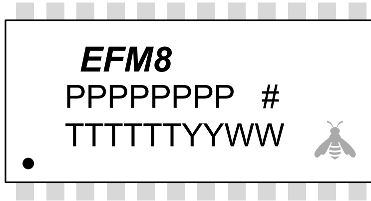
Figure 7.3. QSOP24 Package Marking
