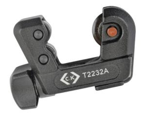
$\sim$  Adjustable pipe cutter for copper, brass, Aluminium and thin walled steel pipe  $\sim$  Replaceable hardened steel cutting blade for long life performance  $\sim$  Black die cast lacquered body for strength and corrosion resistance  $\sim$  Capacity: 3-25 mm Ø Features & Benefits
