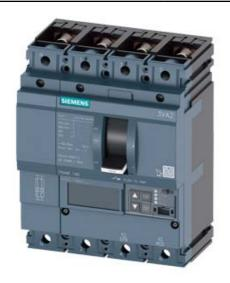
CIRCUIT BREAKER 3VA2 IEC FRAME 160 BREAKING CAPACITY CLASS H ICU=85KA @ 415 V 4POLE, LINE PROTECTION ETU860, LSIG, IN=25A OVERLOAD PROTECTION IR=10A ...25A SHORT CIRCUIT PROTECTION ISD=0,6..10X IN, II=1,5...12X IN NEUTRAL PROTECTION ADJUSTABLE (OFF, UPTO 160%) GROUNDFAULT, SWITCHABLE IG=0,2... 1 X IN, TG=0,050,8MS BUSBAR CONNECTION
