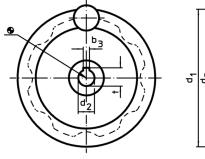
The orientation of the hub keyway may be different than shown in the drawing.
