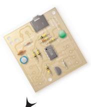
Battery connects here (red wire to '+V', black wire to '0V')
