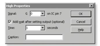
This will light the green LED that is connected to output GO.
