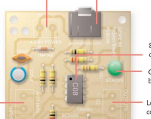
8-pin GENIE microcontroller (the magic bit!)
