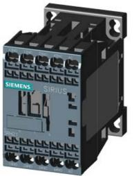
CONTACTOR RELAY, 4NO, AC 110V, 50/60 HZ, W/ FULL-WAVE RECTIFIER, SZ S00, SPRING-LOADED TERMINAL
