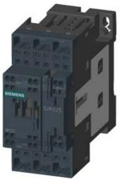
CONTACTOR, AC-3, 15KW/400V, 1NO+1NC, AC(50-60HZ)/DC ACTUAT. AC/DC 21...28V, 3-POLE, SZ S0 SPRING-LOADED TERMINAL
