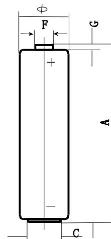
3.6 Capacity: Approximate 1300mAh (10mA, 24h/d, 20°C, e.v.= 0.8V)
