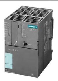
TIM 4R-IE DNP3 COMMUNICATIONS MODULE FOR SIMATIC S7-300, S7-400, PC; WITH TWO RS232/RS485- INTERFACE FOR DNP3- COMMUNICATION VIA CLASSIC WAN NETWORKS AND TWO RJ45-INTERFACES FOR DNP3-COMMUNICATION VIA IPBASED NETWORK (WAN OR LAN)
