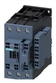
CONTACTOR,AC3:30KW/400V, 2NO+2NC, 230V AC 50HZ, 3-POLE, SIZE S2, SPRING-TYPE TERMINAL LATERAL AUXILIARY CONTACT BLOCK
