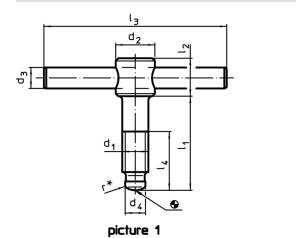
\* to ease assembly the DIN 6304 specification has been completed by r
