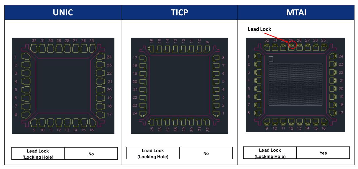
NOTE: Mold compound material fills the <u>lead lock hole</u>, which provides improved protection against moisture penetration along the edge of the leads (pins) of the package.
