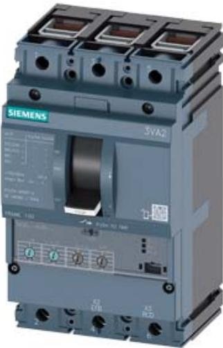
CIRCUIT BREAKER 3VA2 IEC FRAME 100 BREAKING CAPACITY CLASS C ICU=110KA @ 415 V 3POLE, LINE PROTECTION ETU350, LSI, IN=100A OVERLOAD PROTECTION IR=40A ...100A SHORT CIRCUIT PROTECTION ISD=1,5... 10 X IR, II=12 X IN CABLE CONNECTION
