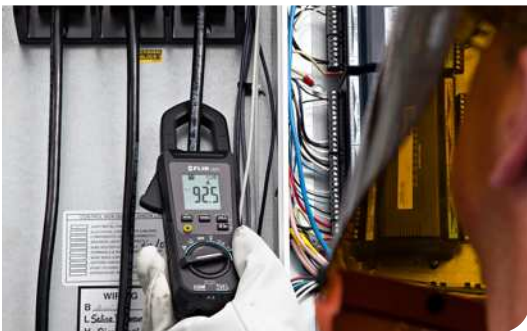
True RMS AC Current up to 600A
