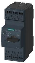
CIRCUIT-BREAKER SZ S0, FOR STARTER COMBINATION, RATED CURRENT 22A, N-RELEASE 286A, SPRING-L. CONNECTION, STANDARD SW. CAPACITY
