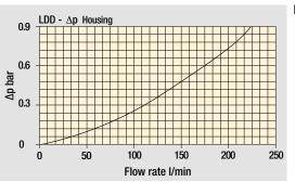
Bypass valve pressure drop
