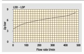
The curves are plotted using mineral oil with density of 0.86 kg/dm<sup>3</sup> in compliance with ISO 3968. Ap varies proportionally with density.
