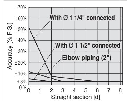
When piping with diameter smaller than the straight section is connected
