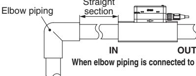
When elbow piping is connected to the IN port
