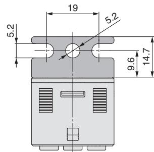
\* Bracket configuration allows for mounting in four orientations.
