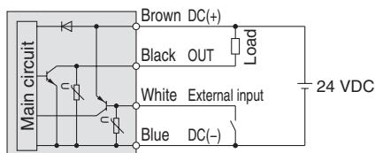
Max. applied voltage: 28 V, Max. load current: 80 mA, Internal voltage drop: 1 V or less
