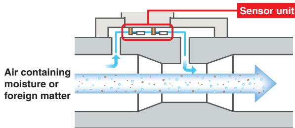
Bypass construction reduces the moist air or foreign matter in contact with the sensor, reducing the accuracy deterioration and damage of the sensor.
