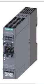
MULTIFUNCTION MODULE; 4 INPUTS AND 2 RELAY OUTPUTS; INPUT VOLTAGE AC/DC 110-240V; MONOSTABLE RELAY OUTPUTS; ANALOG RESIDUAL CURRENT DETECTION WITH RES. CURRENT TRANSFORMER 3UL23 CONNECTION OF A TEMPERATURE SENSOR PT100/PT1000/KTY/NTC; MAXIMUM 1 MULTIFUNCTION MODULE PER SIMOCODE PRO S BASIC DEVICE
