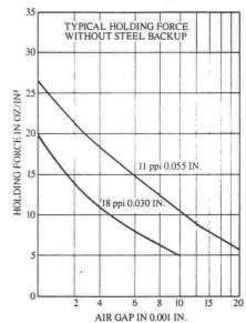
Steel used in magnetic circuit was SAE 1010-1020.
