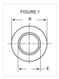
Polyphenylene Sulfide PPS Shoulder Washer. A single gate extension not to exceed  $0.64 \mathrm{mm}$  (0.025) in length is allowable on the outside of all shoulder washers.
