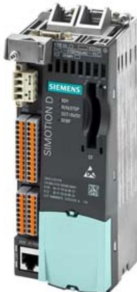
SIMOTION Drive-based Control Unit D410-2 DP/PN; programmable single-axis motion controller with multi-axis option; interfaces: 5 DI, 8 DI/DO, 3 F-DI, 1 F-DO, 1 AI, 1 encoder, 1 DRIVE-CLiQ, 1 PROFIBUS, 2 PROFINET ports, 1 ethernet Note: requires at least SCOUT/firmware V4.3 SP1 HF3
