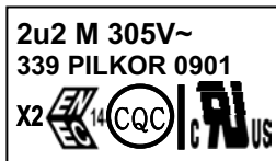
Marking on the top(C > 1uF)
