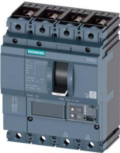
CIRCUIT BREAKER 3VA2 IEC FRAME 160 BREAKING CAPACITY CLASS M ICU=55KA @ 415 V 4POLE, LINE PROTECTION ETU860, LSIG, IN=25A OVERLOAD PROTECTION IR=10A ...25A SHORT CIRCUIT PROTECTION ISD=0,6..10X IN, II=1,5..12X IN NEUTRAL PROTECTION ADJUSTABLE (OFF, UPTO 160%) GROUNDFault, SWITCHABLE IG=0,2... 1 X IN, TG=0,050,8MS BUSBAR CONNECTION
