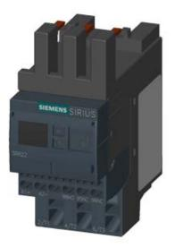
MONITORING RELAY ATTACHABLE TO CONTACTOR 3RT2. SIZE S0 STANDARD, DIGITAL ADJUSTABLE APPARENT/ACTIVE CURRENT MONIT. 4 - 40A, 20-400 HZ, 3-PHASE SUPPLY 24 V AC/DC 1 CO CONTACT, 1 SEMICOND. FOR ALARM AND WARNING MONITORING FOR CURRENT OVERSHOOT/UNDERSHOOT PHASE FAILURE, WIRE BREAK PHASE SEQUENCE FAULT CURRENT BLOCKING CURRENT WARNING AND ALARM THRESHOLDS WITH OR W/O ERROR LOG ON-DELAY 0-99 S SPURIOUS PEAK SUPPR.0-30 S BREAK AFTER FAULT 0-300 MIN SPRING-LOADED CONNECTION
