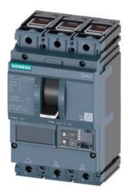
CIRCUIT BREAKER 3VA2 IEC FRAME 160 BREAKING CAPACITY CLASS L ICU=150KA @ 415 V 3POLE, LINE PROTECTION ETU560, LSIG, IN=25A OVERLOAD PROTECTION IR=10A ...25A SHORT CIRCUIT PROTECTION ISD=0,6..10X IN, II=1,5..12X IN NEUTRAL PROTECTION OPTIONAL WITH EXT. CT,UPTO 160% GROUNDFAULT, SWITCHABLE IG=0,2... 1 X IN, TG=0,050,8MS CABLE CONNECTION
