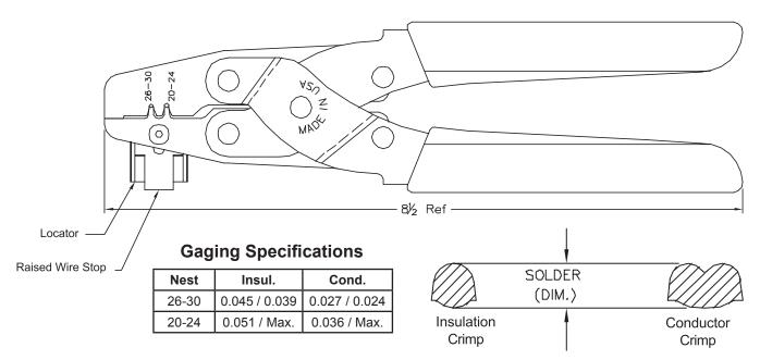
To check tool, insert solid wire solder into cavity nest and crimp to get impressions of shapes shown above. Remove, and measure each shape according to the low and high limits listed in the gaging specification chart.
