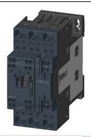
CONTACTOR, AC-3, 11KW/400V, 1NO+1NC, AC 230V 50/60HZ, 3-POLE, SZ S0 SPRING-LOADED TERMINAL
