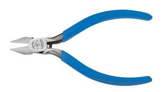
Narrow jaw and hinge for delicate work in tight areas. Sharp pointed nose for precise tip cutting. Spring-loaded action for self-opening. Short jaws and beveled cutting edges permit close cutting of wire. Induction-hardened cutting knives for long life. Hot-riveted joint ensures smooth action and no handle wobble. Plastic-dipped handles for comfort and ease of identification. Custom, US-made tool steel.
