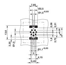
Soldering pad geometry
