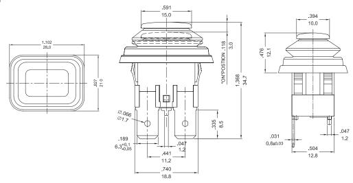
Dimensions : Inches/Millimetres Tolerances ±0.012"/0.3mm
