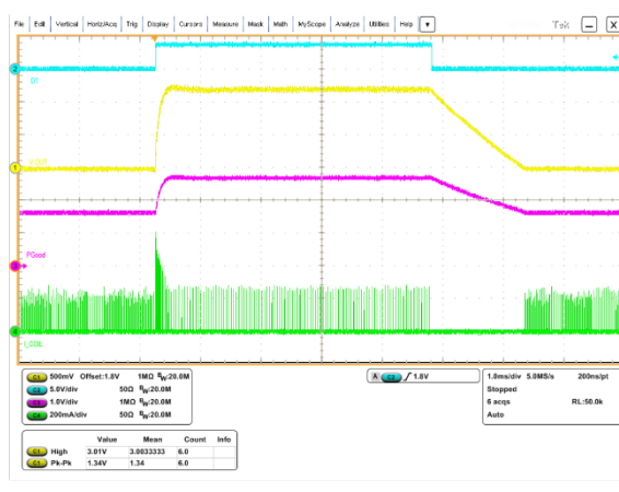
Figure 10. V_{OUT} change, 1.8 V to 3.3 V to 1.8 V, I_{OUT}=5\text{ mA}
