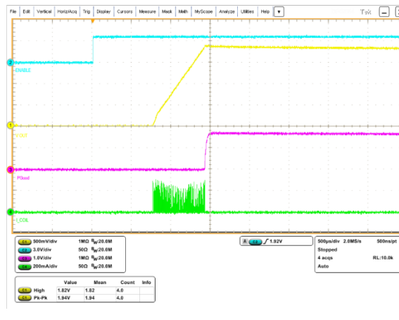
Figure 16. Start-up, V_{IN}=3.6\text{ V} , V_{OUT}=1.8\text{ V} , no load
