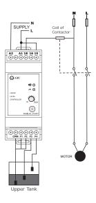
Filling Control (Single level Monitoring with two Sensors)
