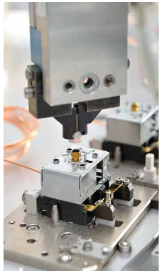
Automated adjustment of thermostats in large-scale series production
